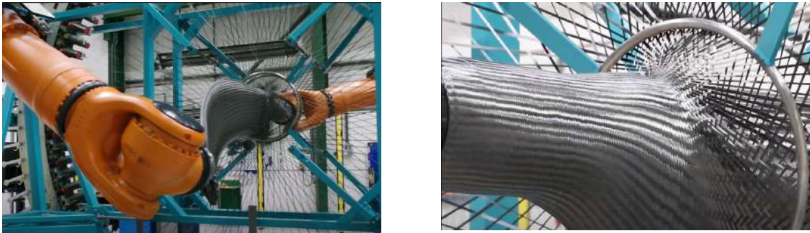
Figure 28.19 Radial braiding technique
