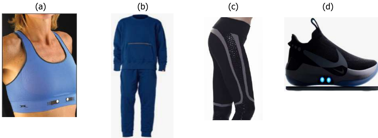
Figure 28.2 Textile sensors based (a) Smart sports bra (b) Sleep lounge suit (c) Yoga pants and (d) Basketball shoes
