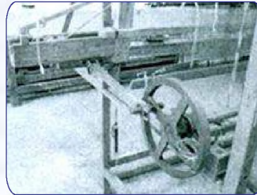
Loom with fly wheel for easy beating and uniform picks in cloth
