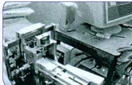
Computerised card punching for getting flawless design cards
